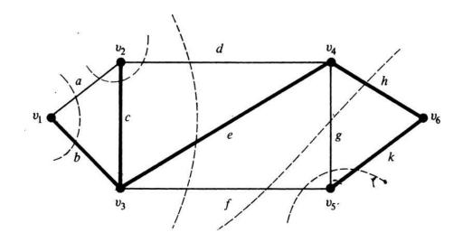
As an example, consider the spanning tree  $\{b, c, e, h, k\}$ , shown in heavy lines, in Fig. 4-3. The fundamental circuit made by chord f is
