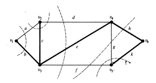
For illustration, in the graph in Fig. 4-3, consider branch *e* of spanning tree {*b*, *c*, *e*, *h*, *k*}. The fundamental cut-set determined by *e* is
